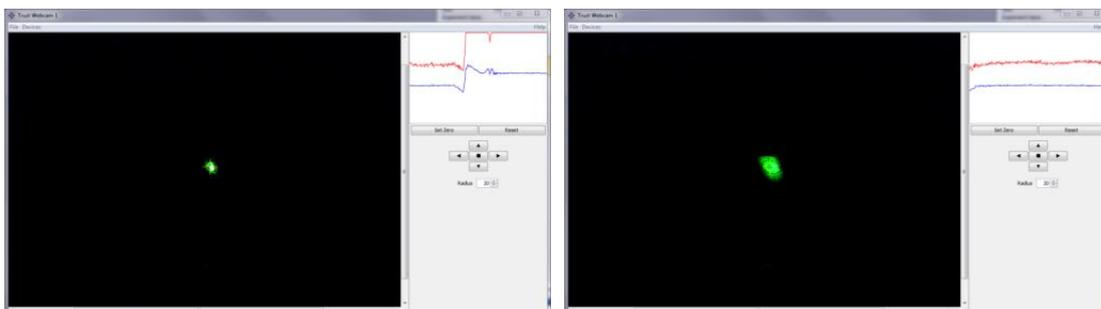
If the spot does not hit the center of the target or is diffuse, proceed with laser alignment.
