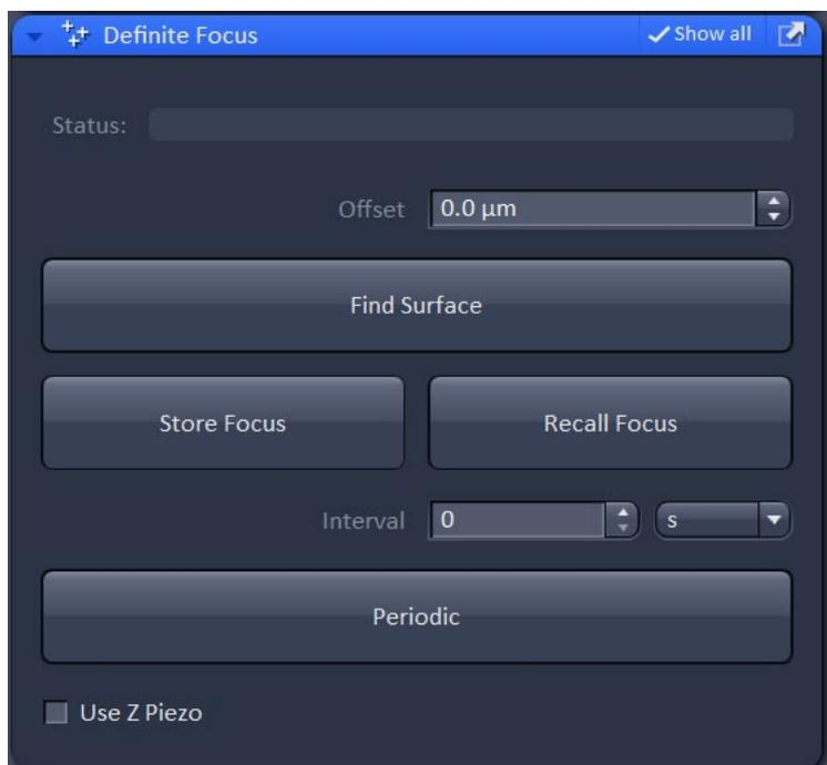
Make sure to have **Show all** activated to be able to see the *Status* bar. If you have moved the objective close to the focus/into the oil you can click *Find Surface* and in the *Status* bar you will see a green blinking message while the *Definite Focus* works. Once it is finished *Status* should read *Reflex found*.
