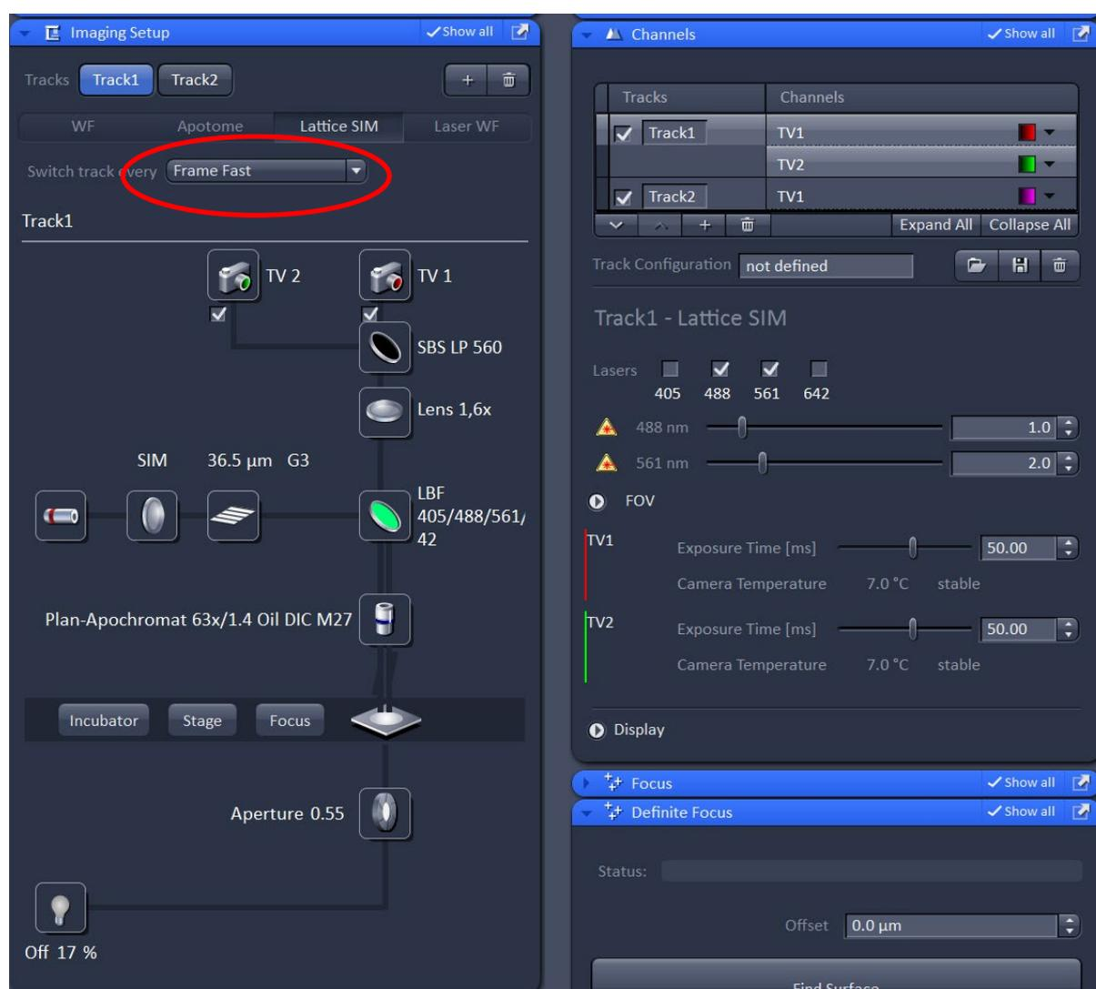
If one does not acquire a z-stack and acquires a single track 2D time-series it is possible to get a higher time resolution by using the so-called *Burst-Mode* in the data processing step.
