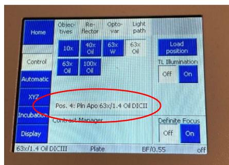
Lattice SIM imaging should only be done with the *63x Oil NA 1.4 lens*. This lens has an NA of 1.4 and is an oil lens as shown in the description on the touchpad.
