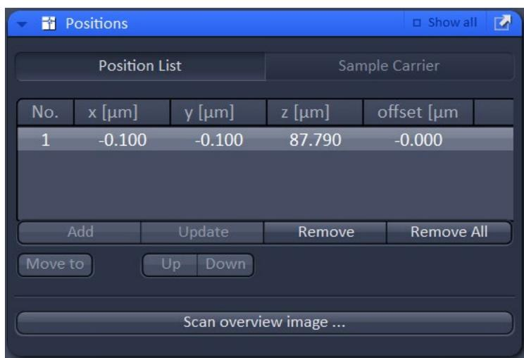
If Positions in the Acquisition tab is activated, this list will be used once you click **Start Experiment** at the top of the Acquisition tab. Each position will be visited automatically and an image will be acquired with the settings you have chosen. If you have set up a z-stack based on a center position, the saved z position will be used as the center of the z-stack.
