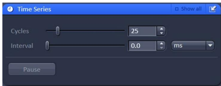
*Interval* refers in this case to the time from the start of one complete image to the start of the next one; in the drop-down box you can choose between ms, s and min.
