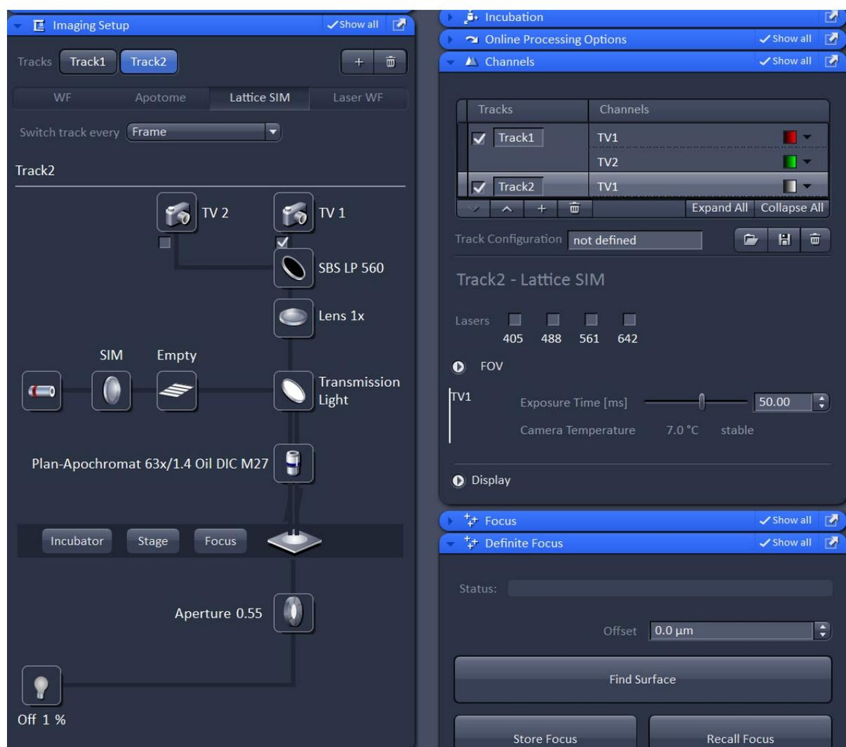
It is possible to add another track with either one or two cameras. Use the small plus symbol on the **Channels** window, right below the list with the tracks to create another track. **But you will need to redefine the light path in the Imaging Setup when doing so!**
