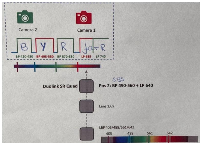
Filter 2, named SBS BP490-560 + LP640 is again a four sections bandpass filter and a beam splitter in one.
