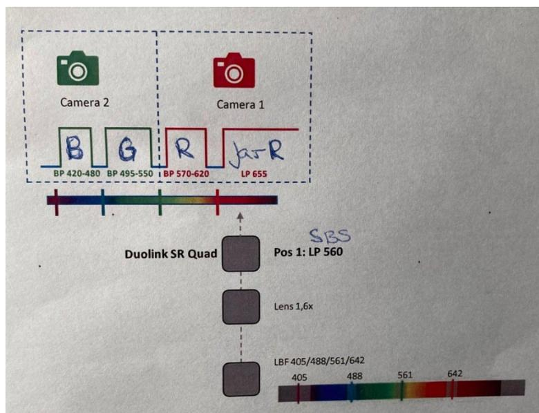
Filter 1, named SBS LP 560, is a bandpass filter with four sections (spectral ranges) and a beam splitter which will direct light below 560nm to Camera 2 and light with a wavelength above 560nm to Camera 1. The four spectral ranges are distributed between the two cameras.
