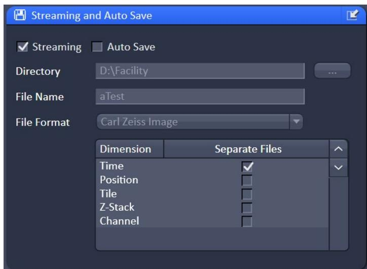
When using the Streaming function, the system will ask you where to save the data after clicking on **Start Experiment**.
