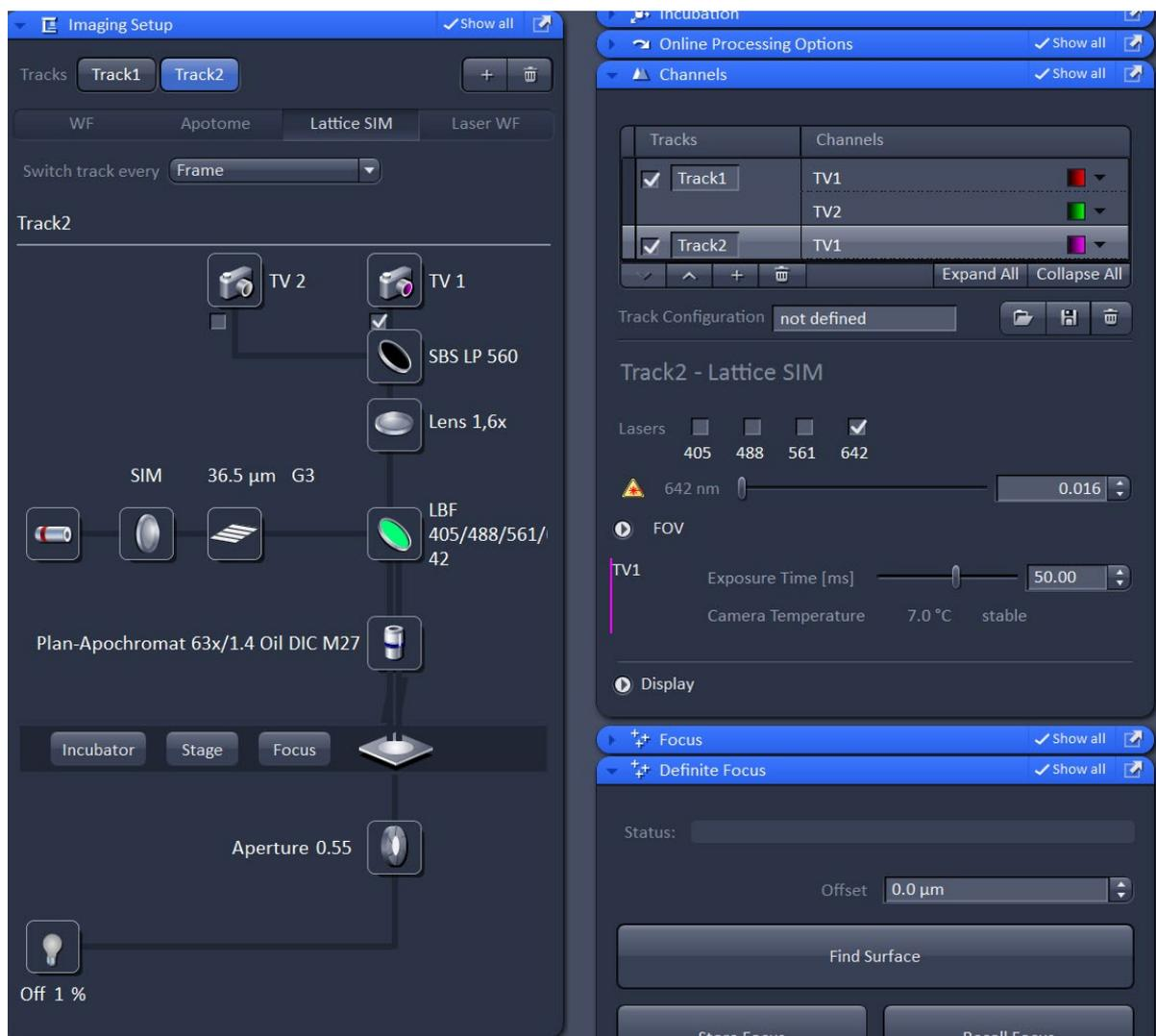
As before, once you choose the excitation laser line the correct Lattice pattern will be put in place. As the pattern is wavelength depend it can be different for different tracks but it is constant for the channels in one track. Again, for the new track you have control of the exposure time and the excitation wavelength power.
