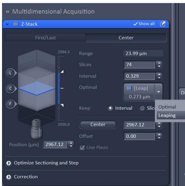
By using **Show all** one has access to two ways to set up the z-stack, as shown to the left: *First/Last* and *Center*.
