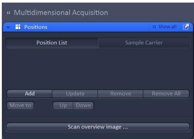
You can make this window freely movable by using the top right white arrow. This allows you to take it over to the Locate tab, where you could use it to find a number of potential imaging positions.
