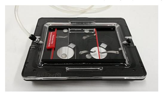
• To level the chamber on the stage, you can adjust 8 screws at the corners of the body of the chamber (using an Allen wrench):
